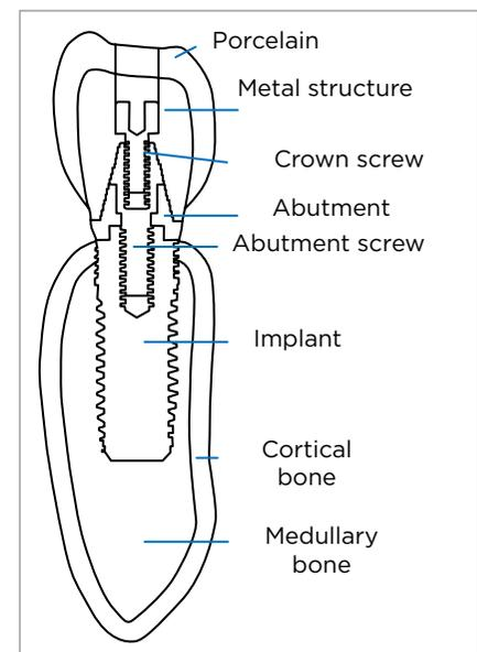
**Figure 2** - CAD drawing of Titamax I implant.
