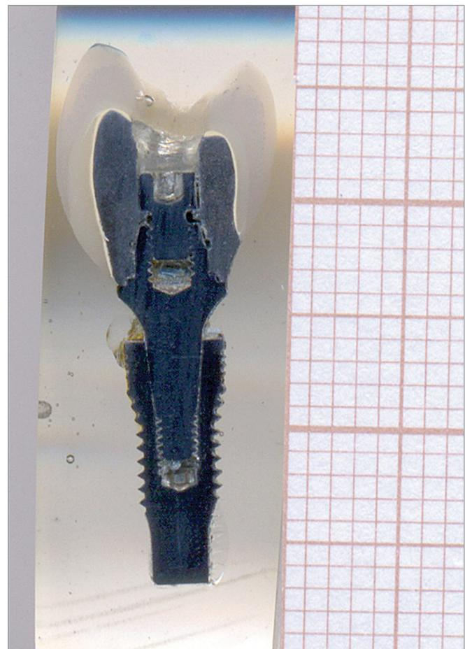
**Figure 1** - Longitudinal section of Morse Taper implant sample.
