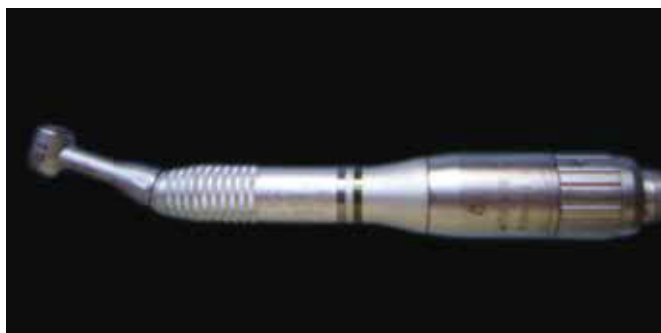
Figure 2. Handpiece Tep E10R 16:1 with head rotation alternating linked to conventional pneumatic micro-motor.
