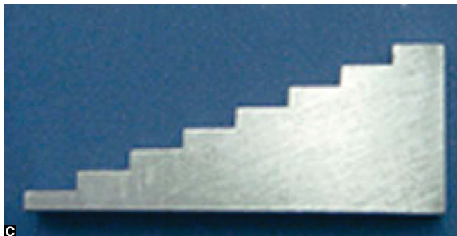
Figure 2. A) X-ray machine positioned, radiographic film, lead plate and step wedge on the Styrofoam; B) Detail of lead and step wedge on the radiographic film; C) Aluminum step wedge.
