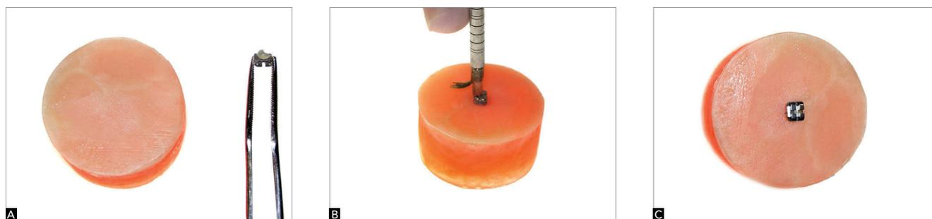
**Figure 1** - Sequence of bonding, **A)** bonding material applied to the base of the bracket, **B)** pressure of 400 gF applied at the moment of bonding to standardize the material thickness, **C)** specimen.
